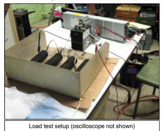
resistors and a very fine antique Weston ammeter for the testing. 73, Lenny W2BVH
